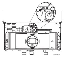
Fig. 32 Gas pressure test port (left tapping)
